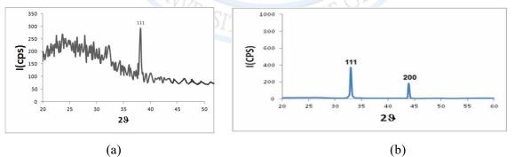
Figure (1): XRD pattern of nano Ag thin film (50 nm)on glass substrate (a) before (b) after sintering.
