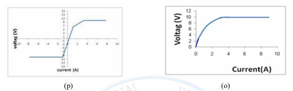
Figuer(7): The I-V characterization of nano Ag thinfilm( o-41,p-46)nm on Si substrat.
