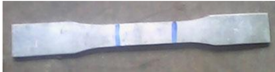
Figure 1. Prepared sample for tensile testing
