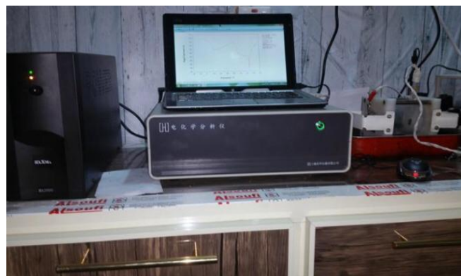
Figure 3. The corrosion test instrument (CHI 604e)
