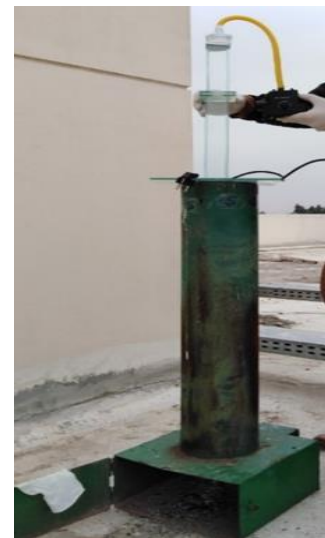
Figure 14. Pilot scale visual permeability test experimental setup
