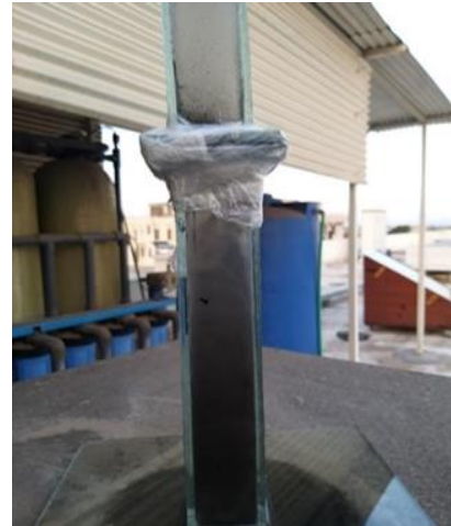
Figure 12. Shows the glass tube where the bottom end is directly connected with chimney, and upper end is connected with vacuum pump. The membrane is placed at the middle of glass tube. Upper part of the glass tube is less blackish compare to lower part as the flue gas is filtered to some extent.
