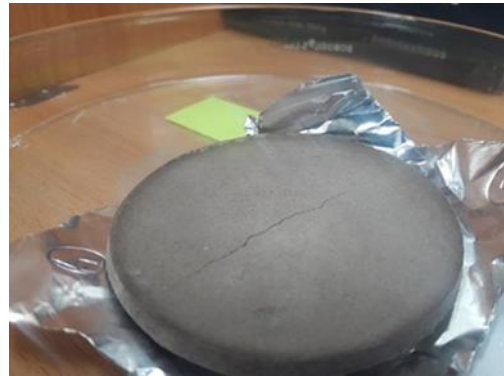
Figure 4. Crack in membrane sample when power supply was stopped to oven during de-moisturization at 105°C for 20 hours.
