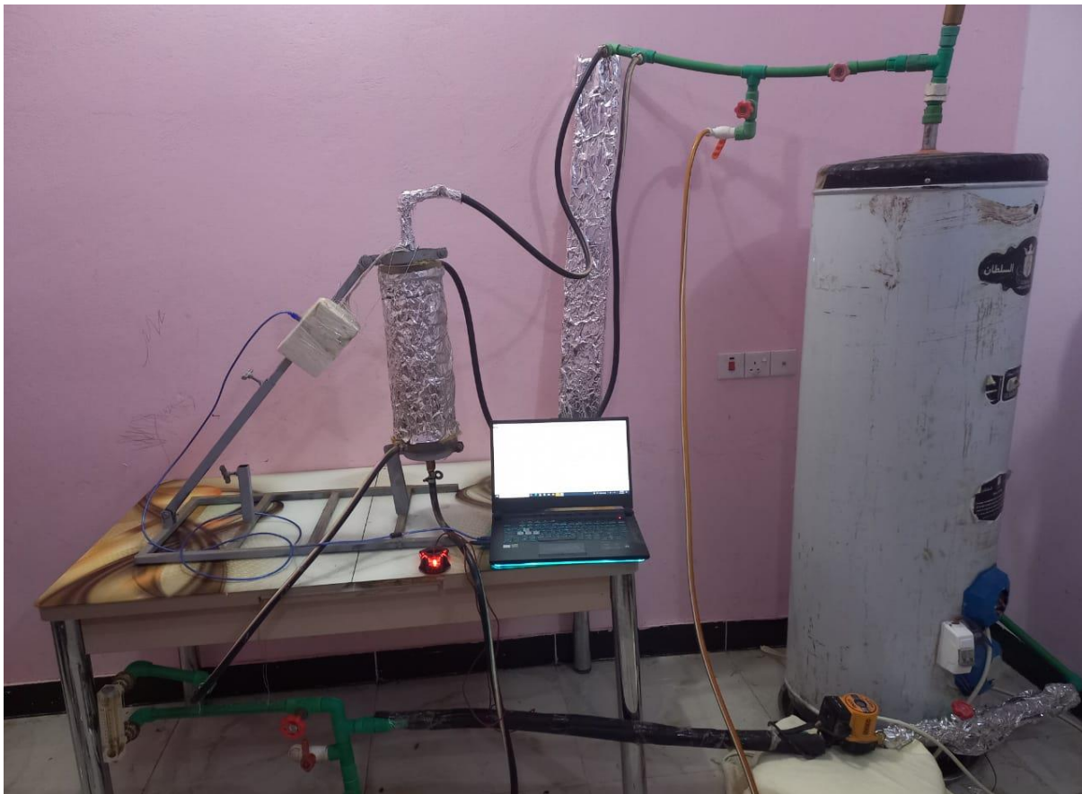
Figure 1. Photograph of LHTES experimental set-up. includes: 1. TTHX, 2. Flow meter, 3. thermocouple, 4. Pump, 5. water tank, 6. Pipes, 7. Valve. 8. Datlogger, 9. Computer, 10. air relieve valve
