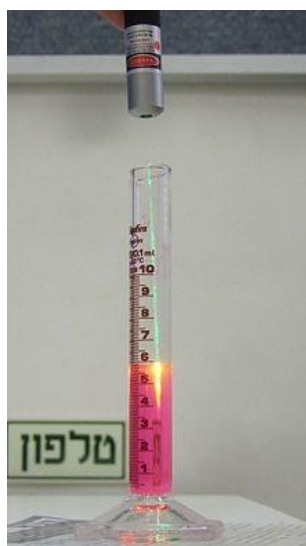
Fig1: A demonstration of the Beer-Lambert law: green laser light in a solution of Rhodamine 6B. The beam radiant power becomes weaker as it passes through the solution.
