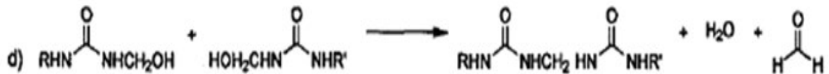
FIGURE 3. Condensation reactions of methylolureas to form (a) methylene bridges between amido nitrogens, (b) methylene ether linkages, and (c) and (d) methylene linkages. Reactions of these types produce higher molecular weight oligomers and polymers.
