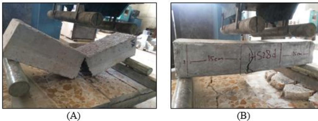
Fig. (6): Crack Pattern of Concrete Specimen under Flexural Test in Sulfate Water Curing; (A) NSC and (B) HFRPC
