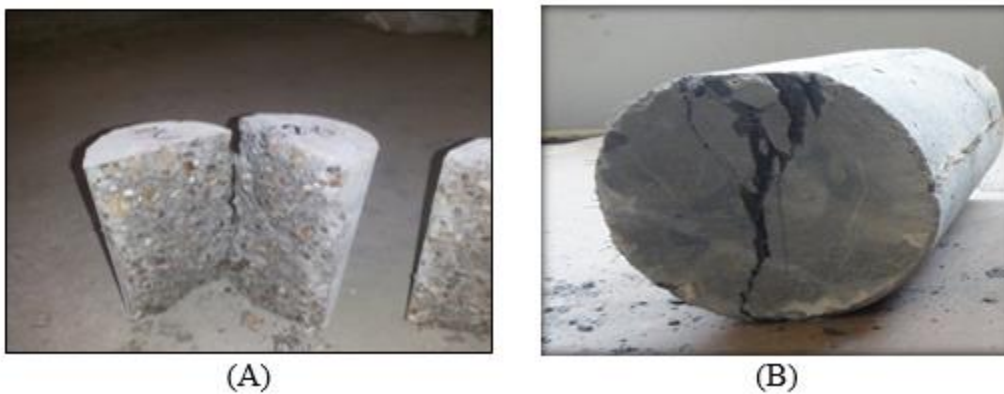
Fig.(8): Crack Pattern Of Concrete Specimen Under Splitting Tensile Test in Sulfate Water Curing ; (A) NSC And (B) HFRPC
