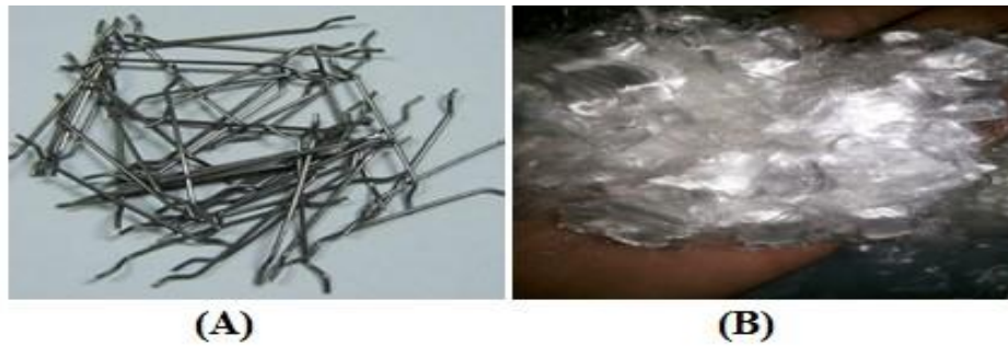
Fig. (1): Photograph of (A) Steel Fiber & (B) Polypropylene Fiber Used In Test
