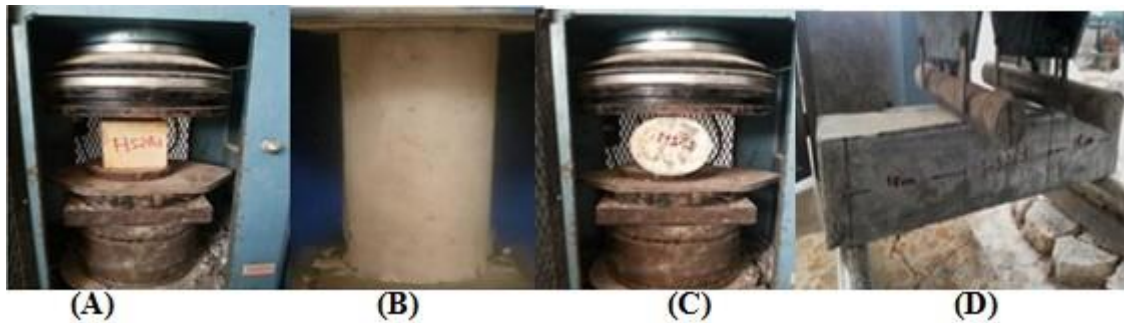
Fig. (5): Specimens under Test where (A) Compressive Strength Test (Cube), (B) Compressive Strength Test (Cylinder), (C) Splitting Tensile Strength Test, (D) Flexural Strength Test
