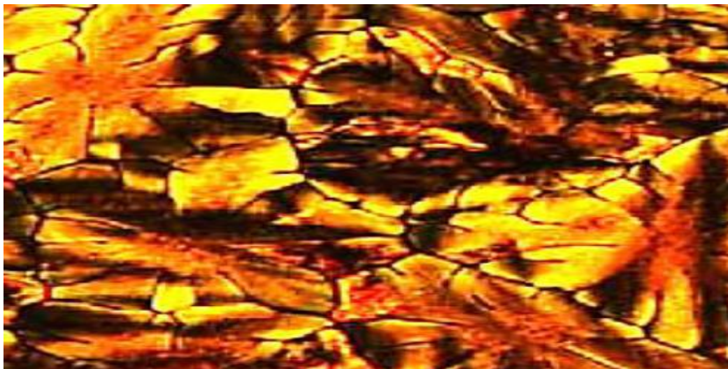
Figure 4: POM textures observed of S_A phase during heating to 309\text{ }^\circ\text{C} of discotic liquid crystal target [A_0]
