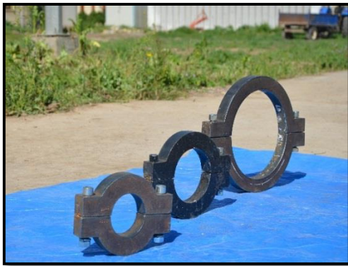
Figure 1: Circular collars of the experimental study.
