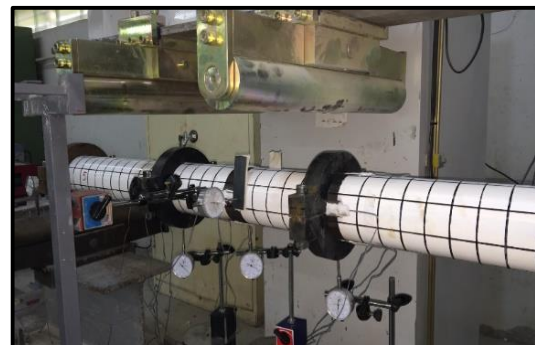
Figure 3: Setup of four-point bending test.
