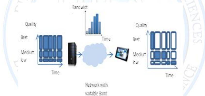
Figure 2: Variable Length Segments Video Streaming
