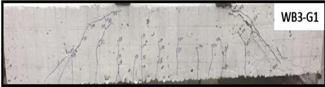
Figure 4. Plate (1) cracking patterns of specimens of Group One
