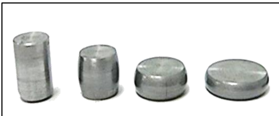
Figure.7 : Compression test of compressed cylindrical samples at 20%, 40%, 50% and 60% reductions.
