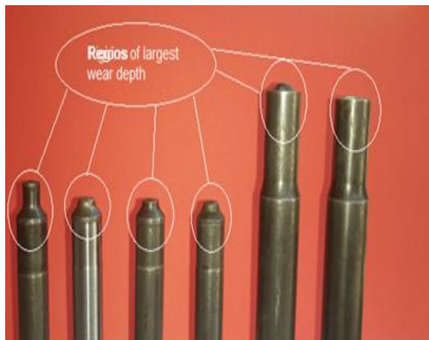
Figure.22: Actual punches for different stages after were scrapped due to wear
