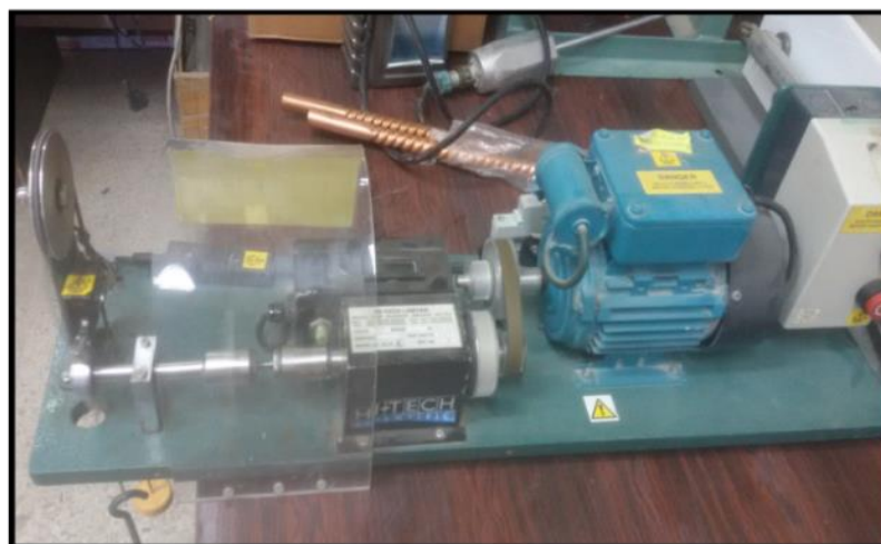
Figure 5 Fatigue testing machine HSM19 (rotating)
