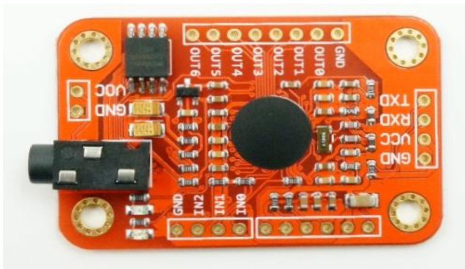
Figure 2: Voice recognition module V3
