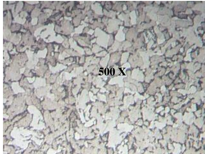
Fig. (2) The surface of carbon steel after Etching
