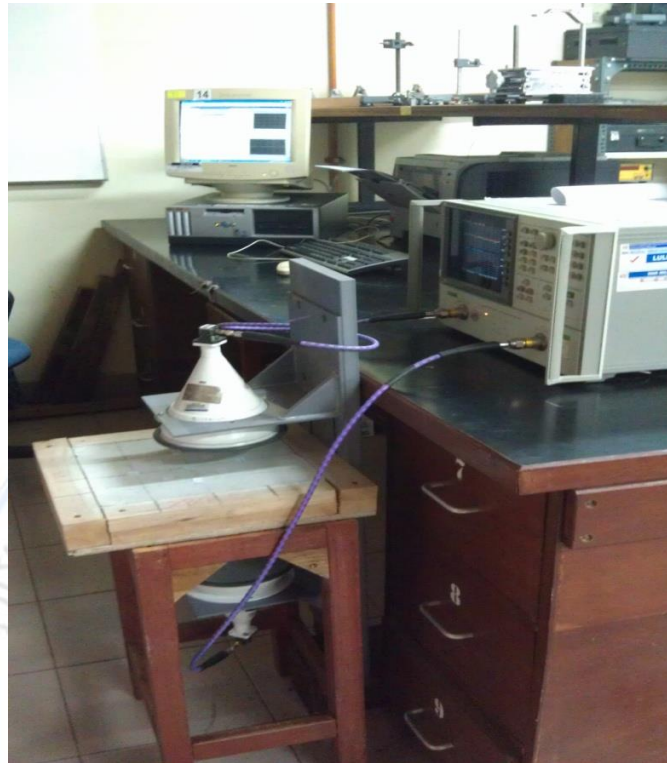
Fig 1: The measurement setup of the free space technique
