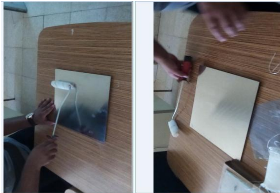
Figure 2. Hand lay-up technique
