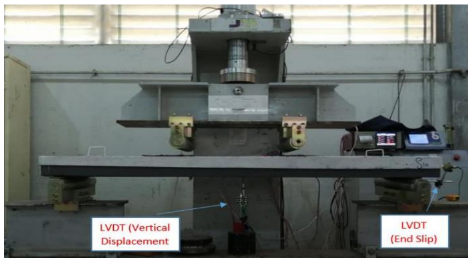
Figure 5. Machine for testing composite slabs
