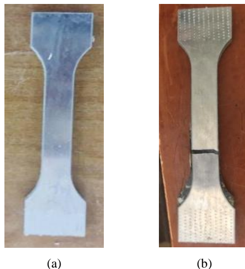
Figure 3. Tensile test sample: (a) before the test (b) after the test
