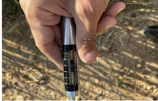
Figure 2. The pocket penetrating soil resistivity meter
