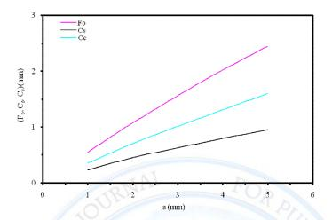
Figure 6: The spherical, chromatic aberration coefficients  $C_s$ ,  $C_c$ , and the objective focal length  $F_o$  as a function of a.
