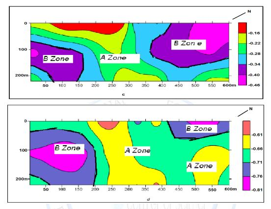
Figure (3) Contour maps for values of material index (I<sub>m</sub>), for a-First layer ,b- Second layer, c-Third layer d- Fourth layer.
