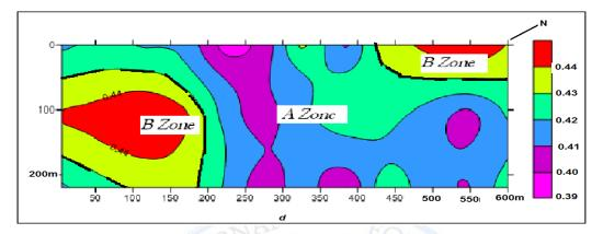
Figure (2) Contour maps for values of Poisson's ratio( $\sigma$ ) for a- First layer ,b- Second layer c-Third layer, d- Fourth layer.
